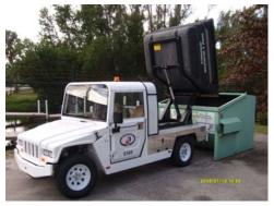
holder and press the up button on the hand held remote switch. Stand back away from the vehicle when lift is in operation. Lift the box until all of the material in box is emptied. Press the down button on the remote switch to lower the box. Never drive the vehicle unless the box is completely lowered. When access to the batteries is needed, lift
