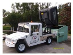
holder and press the up button on the hand held remote switch. Stand back away from the vehicle when lift is in operation. Lift the box until all of the material in box is emptied. Press the down button on the remote switch to lower the box. Never drive the vehicle unless the box is completely lowered. When access to the batteries is needed, lift
